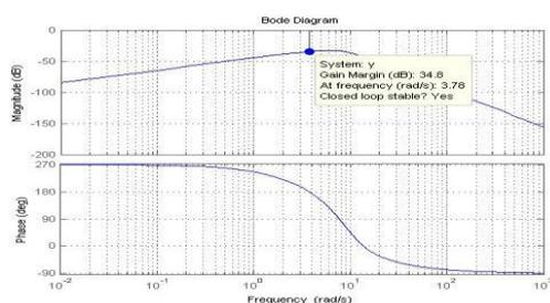
Fig. 11 Bode Plot for SMIB system with optimized PSS parameters using CSO
