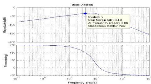
Fig. 10 Bode Plot for SMIB system with optimized PSS parameters using PSO
