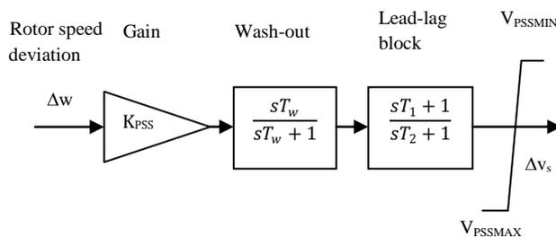
Fig. 2 Basic Power system stabilizer
