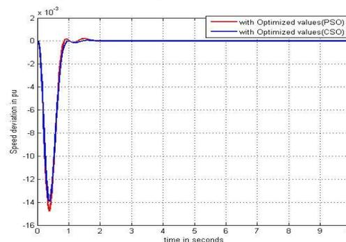
Fig. 9 Speed deviation with PSS
