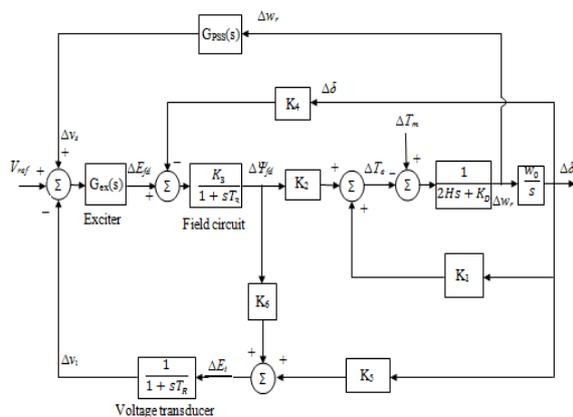
Fig. 1 Block diagram representation with AVR and PSS
